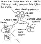
When pumping starts, slightly loosen the flare nut to check of air sucked in Then tighten the flare nut.
